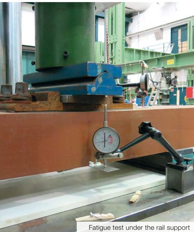
Fatigue test under the rail support
