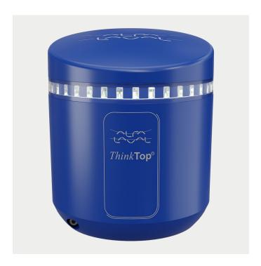
status and condition of the valve position to any programmable logic controller (PLC) system using electrical feedback signals, such as digital, AS-Interface or IO-Link. Light-emitting diodes (LEDs) on the unit provide a 360° visual indication of the valve status, visible from any direction, displaying the current main valve position and any local faults.
